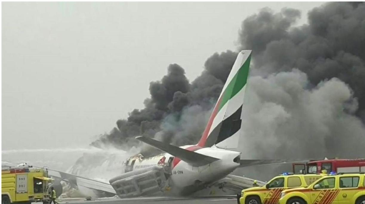
**The initial touchdown and transition from air to ground mode, followed by the lift-off and the changes in the aircraft configuration in the attempted go-around, involved operational modes, logics and inhibitors of a number of systems, including the auto-throttle, the air/ground system, the weather radar, and the GPWS.**
